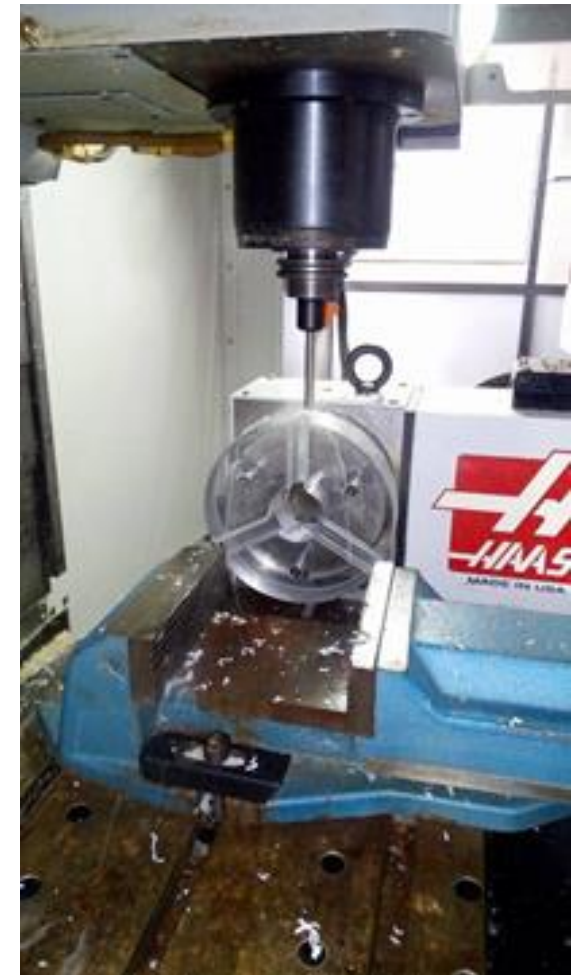
Mounting 4th axis in CNC, own source
